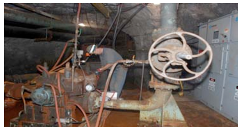
Sanford Lab Infrastructure Technician Bill Heisinger, a former Homestake miner, adjusts a 700-horsepower pump on the 3650 Level at Homestake
