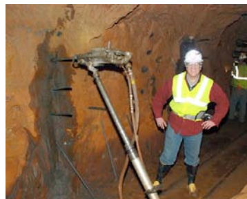
Left: Dr Jose Alonso, Director of Sanford Lab at Homestake, inspects a jackleg drill on the 4550 Level. The jackleg is the iconic tool of hardrock mining. Technicians were using this one to install pins to hold dewatering pipes.
